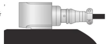
Vibration sensor should be firmly fixed to a flat surface (spot face surface may be needed to be produced and cable anchored to sensor body.)
